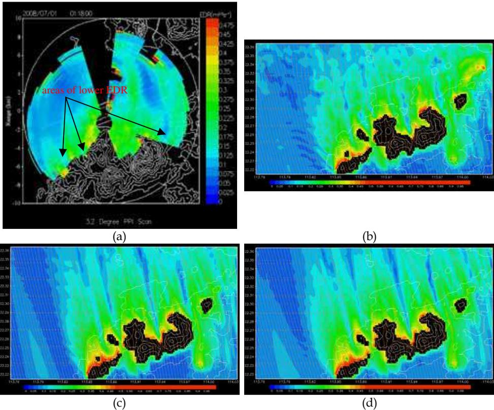
Fig. 6. (a) is the LIDAR-estimated  $EDR^{1/3}$  distribution in the vicinity of the airport at 01:18 UTC, 1 July 2008. The model-simulated results are given in (b), (c) and (d), corresponding to the use of vertical grids with the stretching ratio 1.15, 1.35 and 1.55 respectively.
