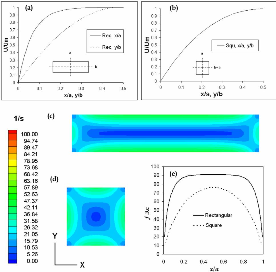
Fig. 5. Non-dimensional velocity profile along two centerlines in (a) rectangular and (b) square flow cell; Strain rate contours ( $1/s$ ) (c) square tube flow cell; (d) rectangular (aspect ratio=5) tube flow cell; (e) Non-dimensional shear stress at the base of square and rectangular flow cells (Salek & Martinuzzi, 2007, ASME)
