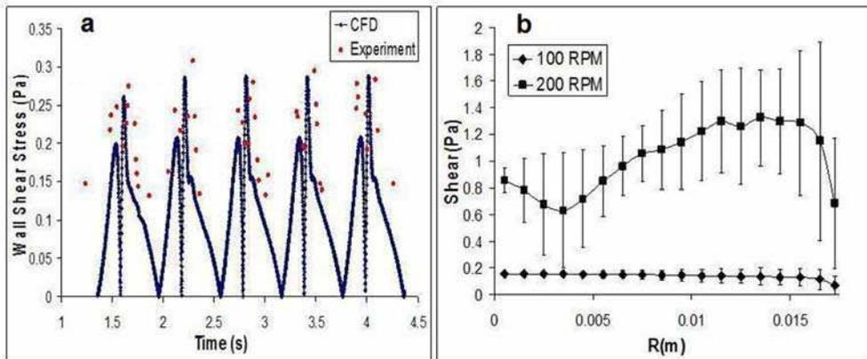
Fig. 7. (a) Time series of numerical and experimental wall shear stress component magnitude for 5 cycles at  $r=12\text{mm}$  from the center and 100 RPM; (b) Radial distribution of the mean wall shear stress magnitude at 100 and 200 RPM (Reprinted from (Salek et al., 2010a), IEEE)
