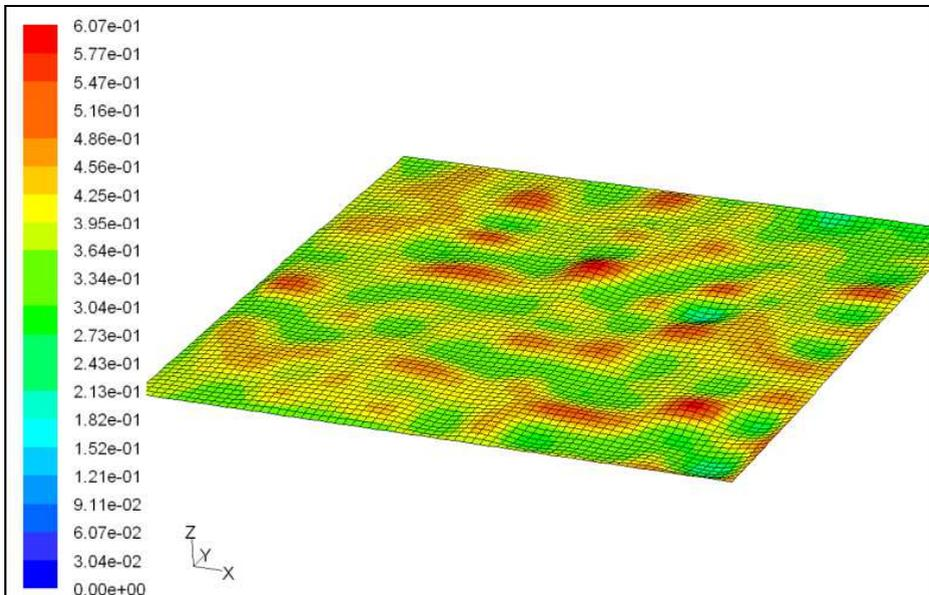
Fig. 3. Wall shear stress distribution over the reconstructed Endothelial Cells in a  $\mu$ -channel as determined by CFD (unit is in Pa). Reprinted from (Dol et al., 2010), ASME. Note that shear stress distribution correlates well with local roughness height
