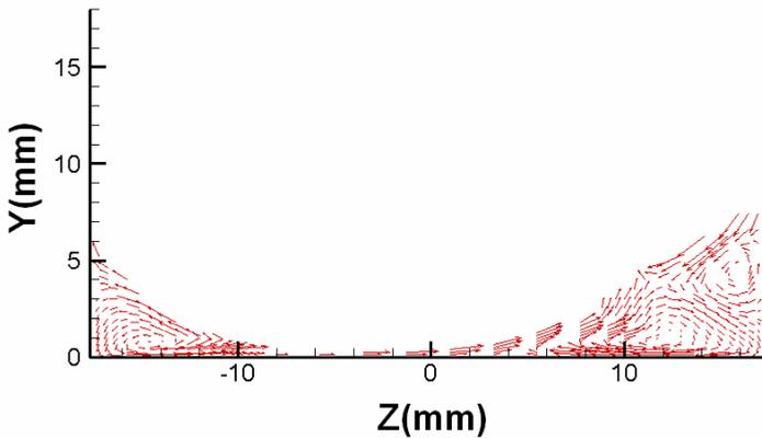
Fig. 9. Vector plots of flow in liquid phase with free-surface inside an individual well, 200rpm, 4ml
