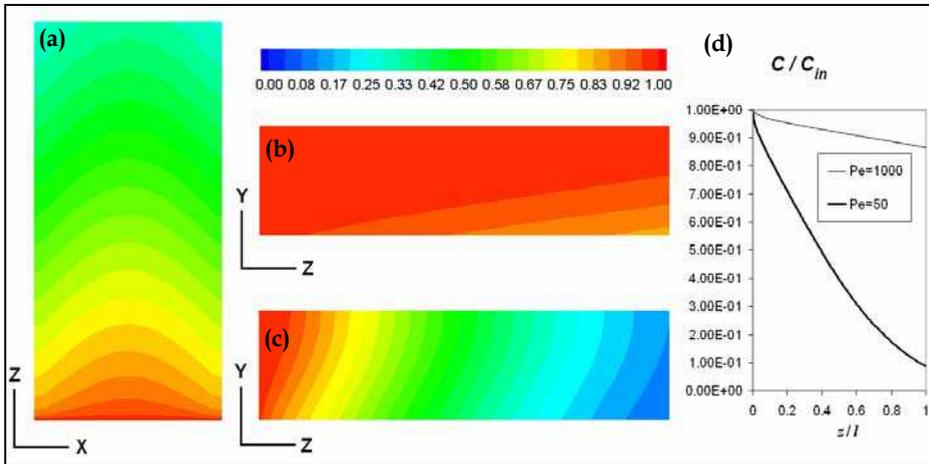
Fig. 6. Substrate concentration in the square flow cell (a) at the base at  $Pe=100$ ; (b) and (c) at the mid plane at  $Pe= 1000$  and  $50$  respectively; (d) at the base (Salek & Martinuzzi, 2007, ASME)
