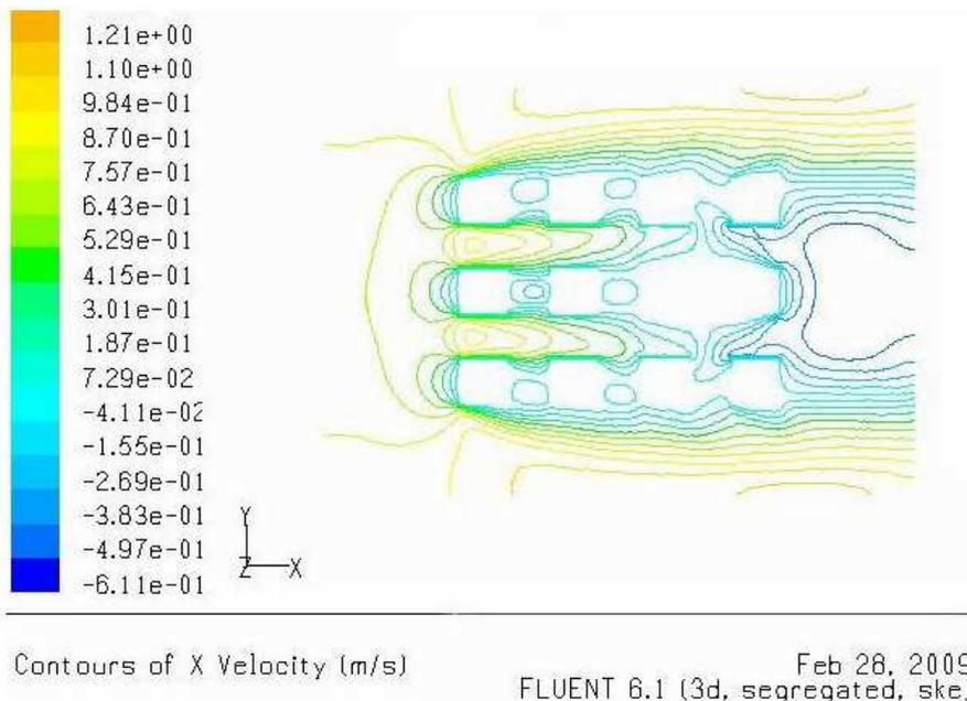
Fig. 8. Velocity distribution in x-y plane at  $z = 0.5$  and a Reynolds number is  $9.0 \times 10^5$
