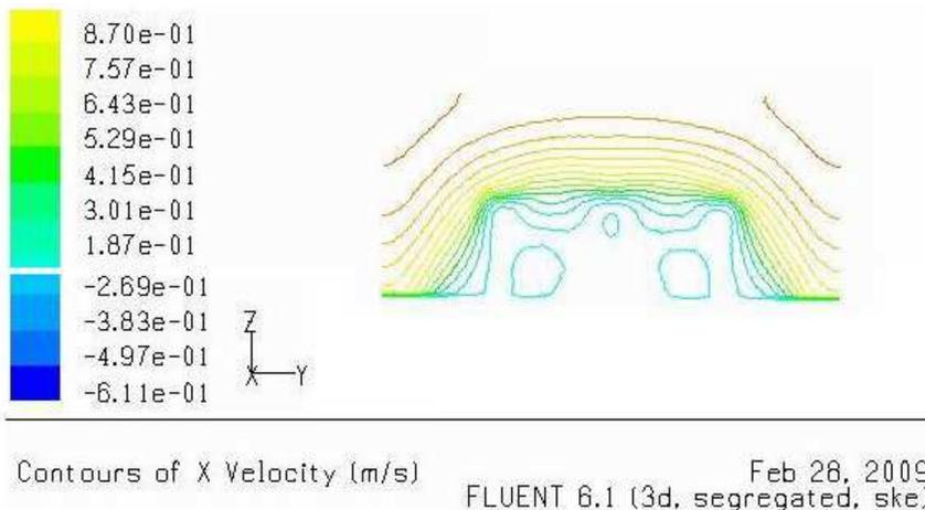
Fig. 4. Velocity distribution in y-z plane at  $x = 2.0$  and a Reynolds number is  $9.0 \times 10^5$
