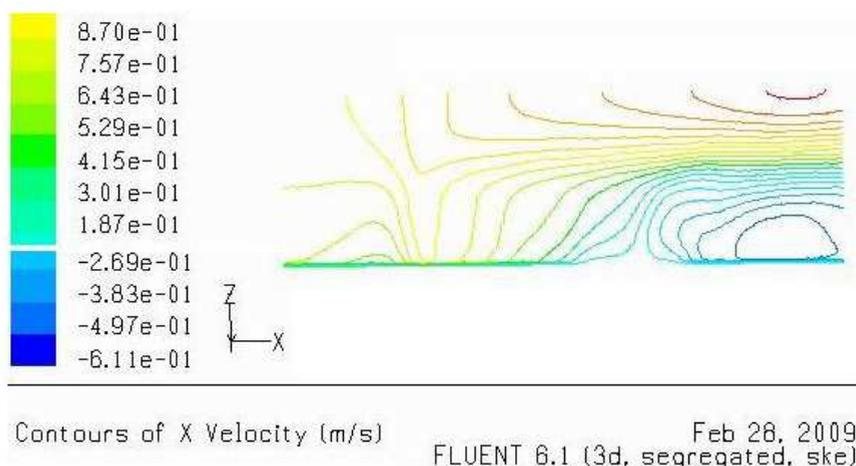
Fig. 6. Velocity distribution in x-z plane at  $y = 1.0$  and a Reynolds number is  $9.0 \times 10^5$
