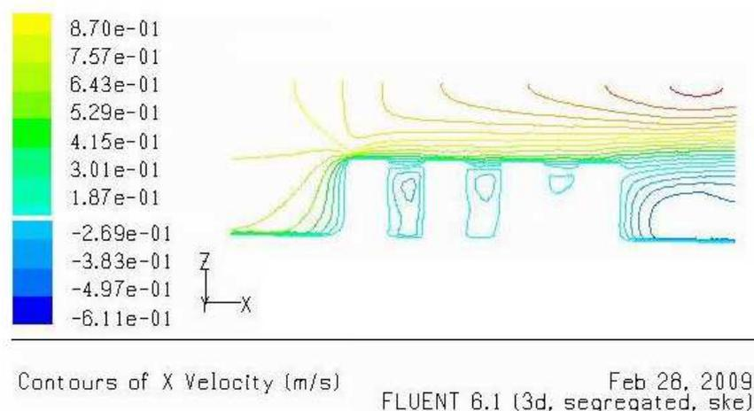
Fig. 5. Velocity distribution in x-z plane at  $y = 0.0$  and a Reynolds number is  $9.0 \times 10^5$
