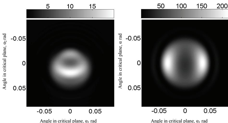
Fig. 9. Gain factors of harmonic disturbances a) fundamental and b) second harmonic waves. Calculated for 0.5mm KDP crystal and intensity 4.5TW/cm<sup>2</sup>, angle of strong wave's propagation is optimal according to (2).
