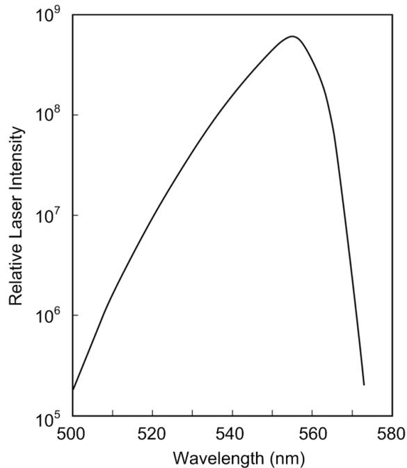
Fig. 8. Tuning curve of the transversely-excited coumarin 545 tetramethyl dye laser. The tuning range of the emission is  $501 \leq \lambda \leq 574$  nm and the dynamic range of its output intensity span approximately four orders of magnitude (from Duarte et al. (2006)).
