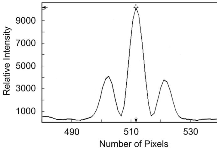
Fig. 5. Double-slit interferogram of the emission from the  $\lambda \approx 543.30$  nm narrow-linewidth He-Ne laser using the interferometric configuration depicted in Figure 1b. The visibility recorded at  $z = 50$  mm is  $\mathcal{V} \approx 0.95$  while the measure laser linewidth is  $\Delta\lambda \approx 0.001$  nm. Each pixel is  $25 \mu\text{m}$  wide (from Duarte et al. (2005)).
