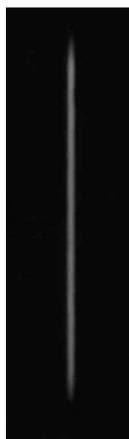
Fig. 9. Black and white silver halide photograph of the near-Gaussian emission beam, from the interferometric emitter (DICOS), recorder under nanosecond pulsed excitation at  $\sim 10$  kV per pulse. The corresponding excitation current density is  $\sim 190$  A/cm<sup>2</sup> (from Duarte (2008)).
