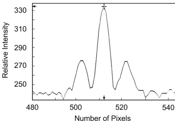
Fig. 4. Double-slit interferogram of the emission from the interferometric emitter using the configuration depicted in Figure 1b. The visibility recorded at  $z = 50$  mm is  $\psi \approx 0.9$  leading to an interferometrically determined linewidth of  $\Delta\lambda \approx 10.5$  nm. Each pixel is 25  $\mu\text{m}$  wide (from Duarte et al. (2005)).
