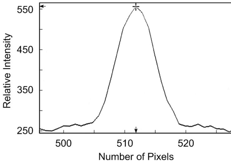
Fig. 3. Digital profile of the near-Gaussian emission beam, with a measured divergence  $\sim 1.1$  times its diffraction limit, recorded at  $z = 340$  mm. Each pixel is  $25 \mu\text{m}$  wide (from Duarte et al. (2005)).
