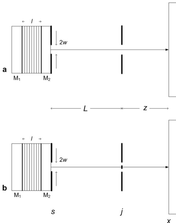
Fig. 1. (a) Electrically-pumped organic semiconductor interferometric emitter depicting the sub micrometer cavity with  $l \approx 300$  nm.  $M_1$  is a total reflector and  $M_2$  is a low reflectivity output coupler (see text). (b) Double-slit interferometric configuration used to determine the coherence of the emission. The slits are  $50 \mu\text{m}$  wide separated by  $50 \mu\text{m}$ . The distance to the interferometric plane is  $z$  (from Duarte (2008)).
