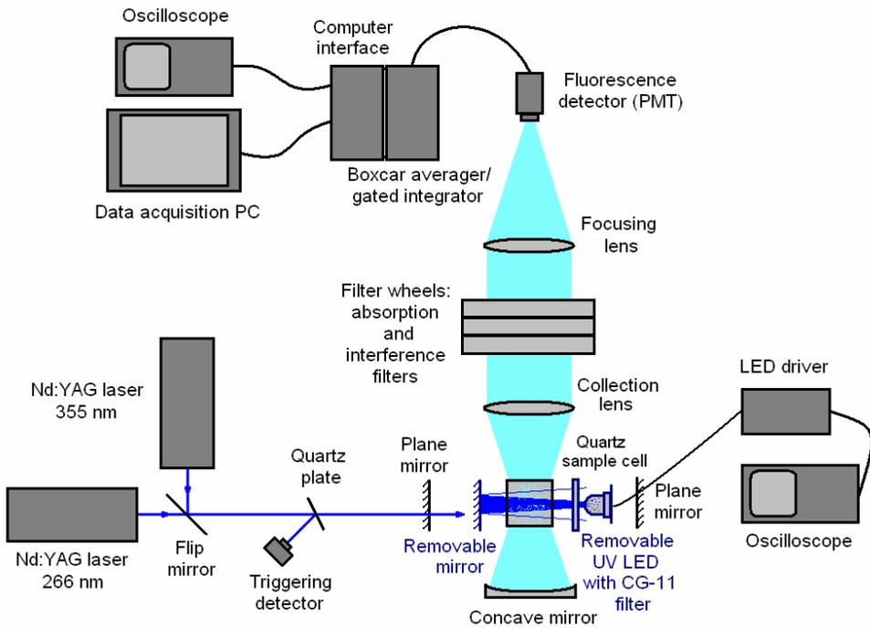
Fig. 2. Schematic diagram of the experimental apparatus
