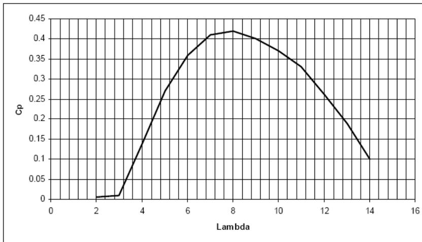
Fig. 7. Power coefficient  $C_p$  curve versus  $\lambda$
