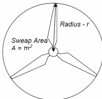
Fig. 4. Swept area of the wind turbine
