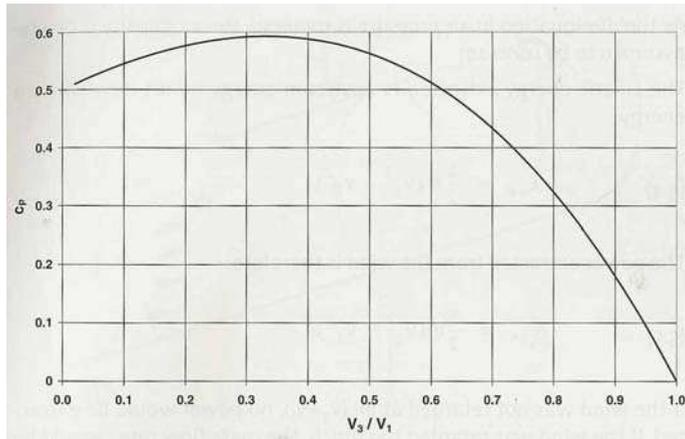
Fig. 6. Power coefficients  $C_p$  versus  $V_3/V_1$  ratio
