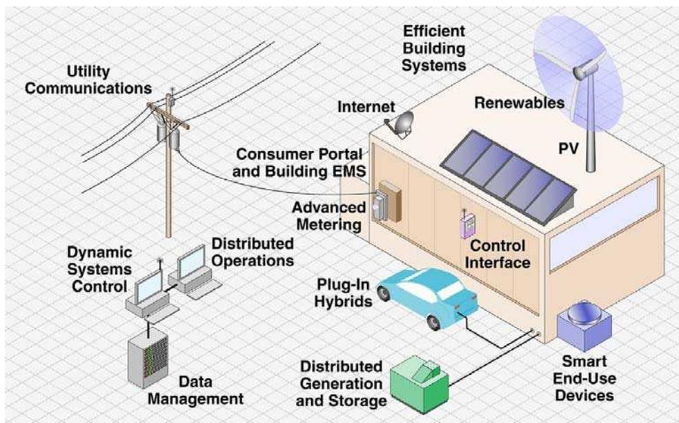
Fig. 4. A schematic of smart grid utilization <sup>5</sup>
