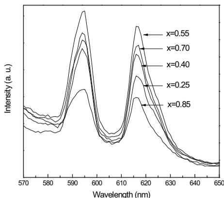
Fig. 5. PL emission spectra of  $\text{Bi}_{4-x}\text{Eu}_x\text{Ti}_3\text{O}_{12}$  thin films on STO (100) substrates ( $\lambda_{\text{ex}}=350$  nm). Ref. [48] Ruan, K.B., et al., J. Appl. Phys., 104, 036101 (2008). Copyright American Institute of Physics (2008)
