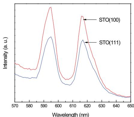
Fig. 6. PL emission spectra of  $\text{Bi}_{3.45}\text{Eu}_{0.55}\text{Ti}_3\text{O}_{12}$  thin films prepared on STO (100) and STO (111) substrates. Ref. [48] Ruan, K.B., et al., J. Appl. Phys., 104, 036101 (2008). Copyright American Institute of Physics (2008)
