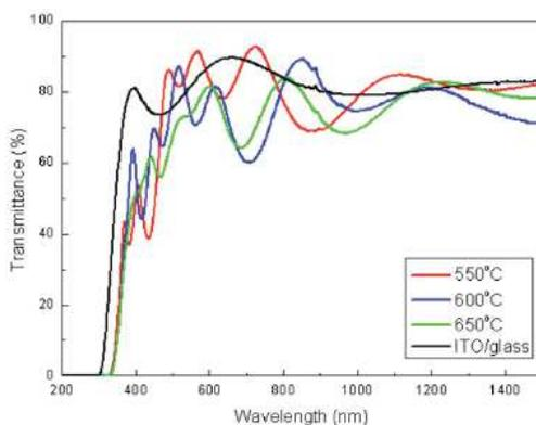
Fig. 1. Optic transmittance of BEuT ( $x=0.85$ ) thin films annealed at different temperatures. From Ref. [36] Ruan, K.B., et al., *J. Appl. Phys.*, 103, 074101 (2008). Copyright American Institute of Physics (2008)
