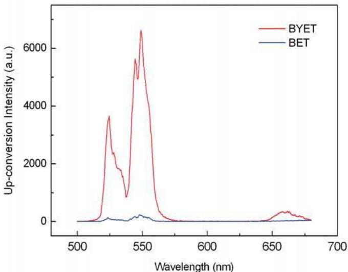
Fig. 11. Up-conversion luminescence spectra of BET and BYET thin films on fused silica substrates pumped by 980 nm. From Ref. [65] Gao, F., et al., *J. Appl. Phys.*, 106, 126104 (2009). Copyright American Institute of Physics (2009)
