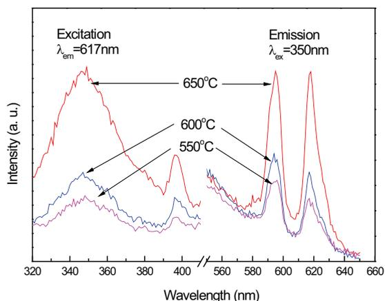
Fig. 2. Excitation and emission spectra of BEuT ( $x=0.85$ ) thin films annealed at different temperatures. From Ref. [36] Ruan, K.B., et al., *J. Appl. Phys.*, 103, 074101 (2008). Copyright American Institute of Physics (2008)
