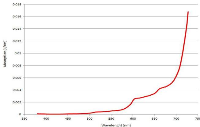
Fig. 2. Underwater Attenuation of Light from experimental data
