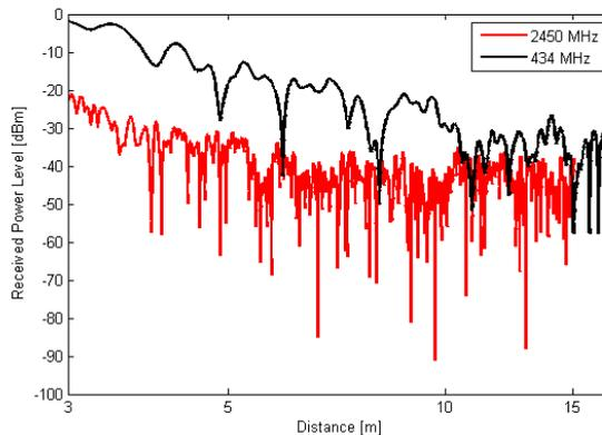
Fig. 1.4. Typical measurement at 434 MHz and 2450 MHz.
