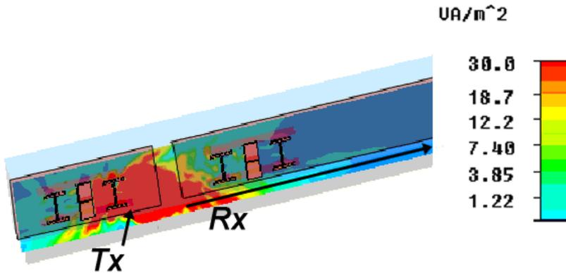
Fig. 1.5. A simulation result showing the field strength. Visualizing plane is approximately at a height of 0.5 m above ground level.
