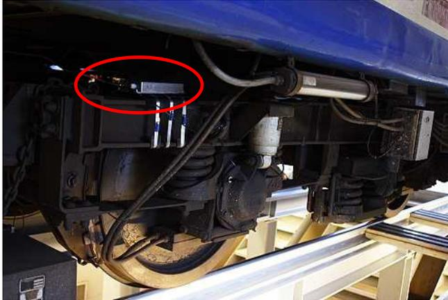
Fig 1.1 The position of the wireless sensor.
