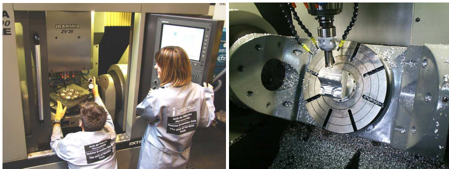
Fig. 3. a) Students learning the five-axis machining technology. b) Component made by five-axis milling
