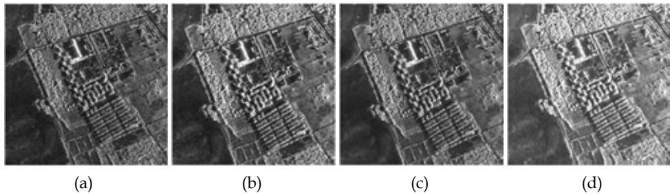
Fig. 8. (a)Original image of Cairo, Egypt (©DLR). (b) MAP-MBD despeckled (c) MAP-ABM despeckled. (d) MAP-GGMRF despeckled.
