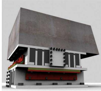
Fig. 2.10. SERB SITON RP 1000 x 1000 rolling or sliding capsulated device
