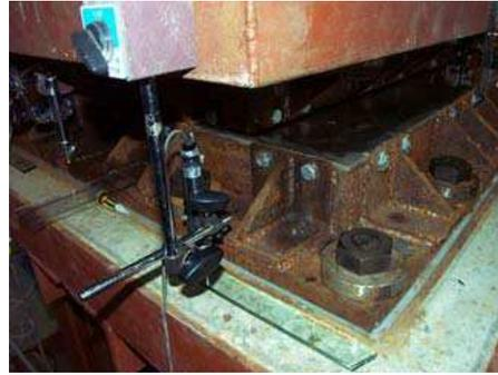
Fig. 2.9. SERB - SITON LP 800 x 800 capsulated isolation device with sliding on plane surfaces
