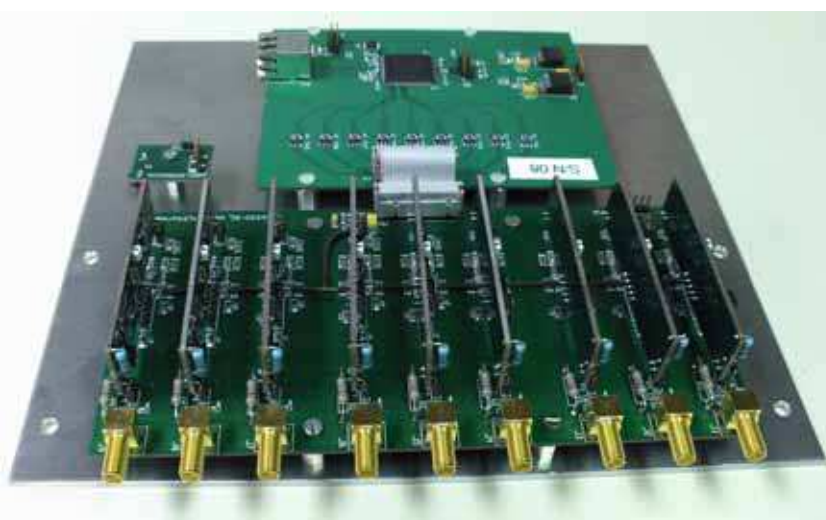
Fig. 12. Electronics for one detector module (Front: Single channel boards on the carrier board; Back: Digitizing board; Small circuit left of digitizing board: 1-wire temperature sensor).
