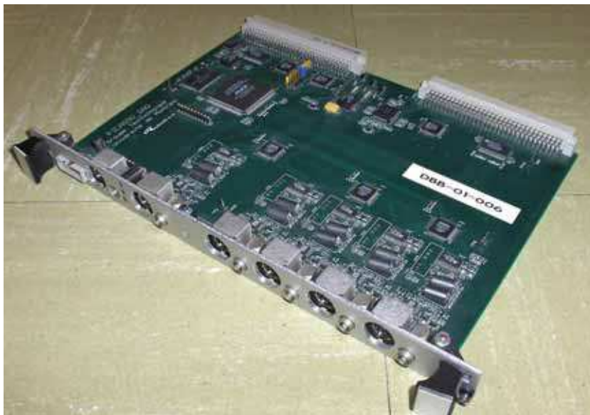
Fig. 4. Previously used VME module for PICASSO data acquisition.
