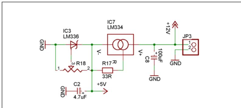
Fig. 6. Power supply for A/D converter schematics
