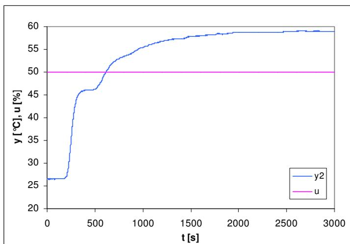
Fig. 18. Measured step response of heating plant model
