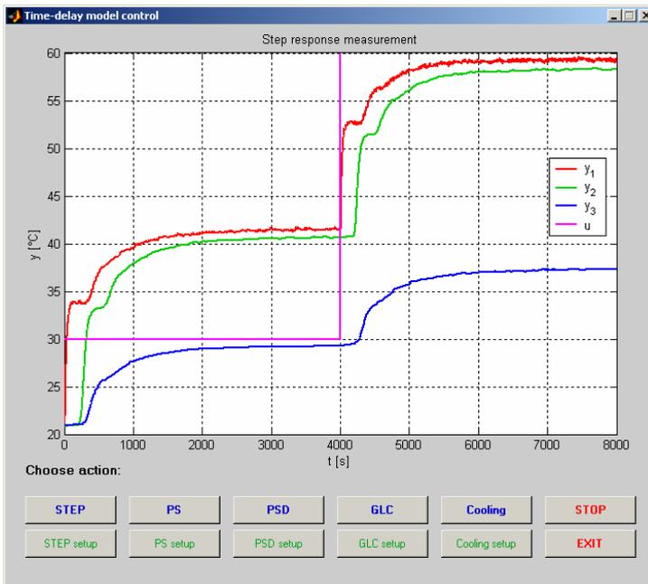
Fig. 17. Heating plant model control application for Matlab 6.5
