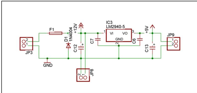
Fig. 5. Power supply for digital circuits schematic
