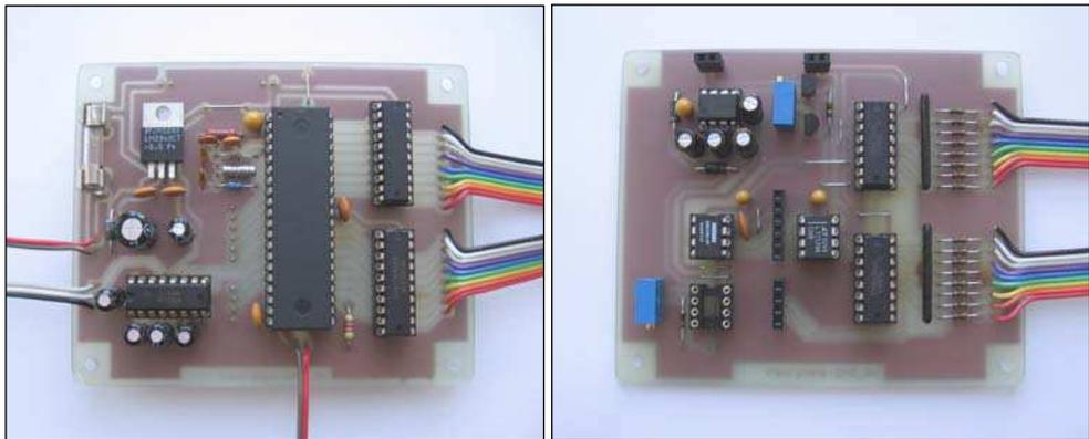
Fig. 8. Finalized DAQ device printed circuit boards
