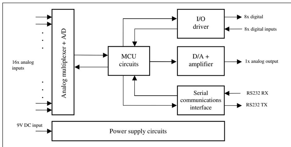
Fig. 1. Block diagram of the DAQ device
