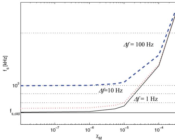
Fig. 2. Optimal sample rate versus clock accuracy, for different values of  $\Delta f$ . The bandpass signal under test has a bandwidth  $B = 140$  kHz and a carrier frequency  $f_c = 595.121$  MHz. The value chosen for  $p$  is 10.
