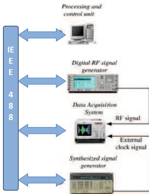
Fig. 7. Measurement station.
