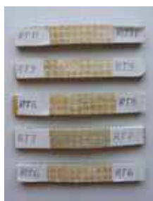
Fig. 19. Flexural specimens made of E-glass EWR145 / fir wood flour / polyester Colpoly 7233 after flexural test
