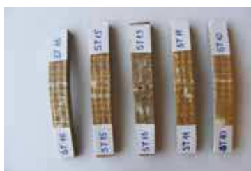
Fig. 18. Flexural specimens made of E-glass EWR145 / oak wood flour / polyester Colpoly 7233 after flexural test
