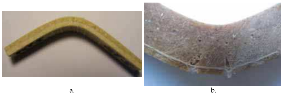
Fig. 32. Failure area occurred during flexural tests in case of the specimens additionally reinforced with wood flour: a. fir wood flour; b. oak wood flour
