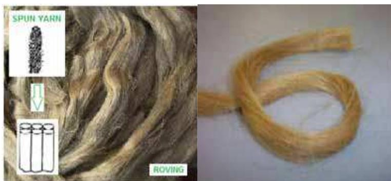
Fig. 10. Hemp and flax fibre rovings
