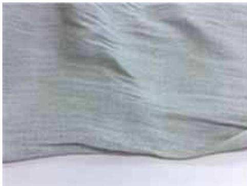
Fig. 28. Weaved fabric (0/ 90) with twisted yarns
