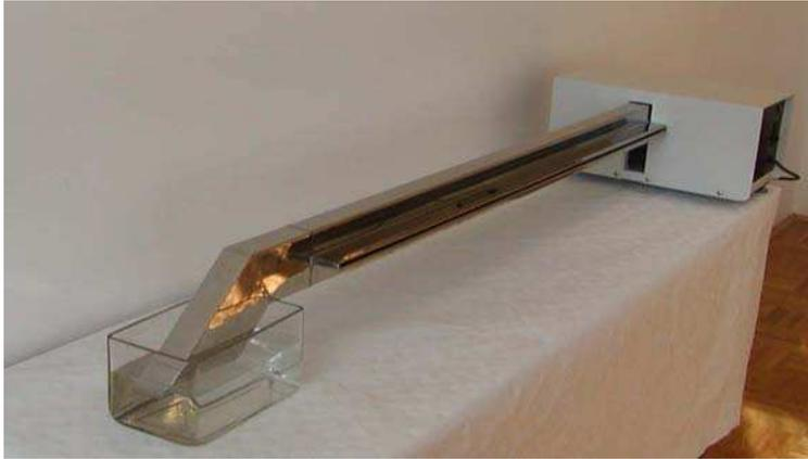
Fig. 13. The modular microwave unit
