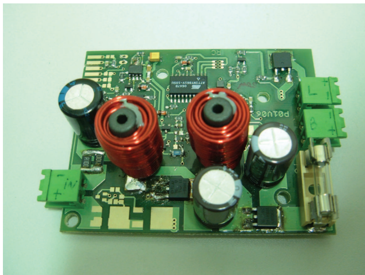
Fig. 9. Photo of the MPPT and battery charger prototype board.
