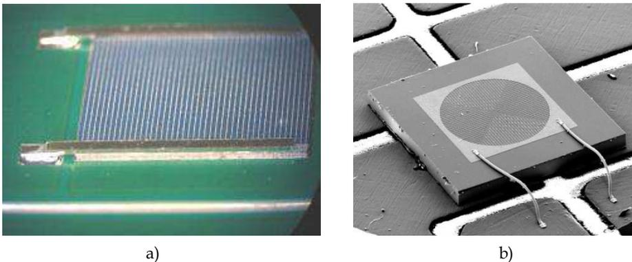
Fig. 12. CPV solar cells assembled on substrates: a) soldered silicon solar cell (Courtesy of CPower Srl); b) solar cell of 1mm<sup>2</sup> assembled with chip on board technology (Courtesy of CRP - Centro Ricerche Plast-ottica)
