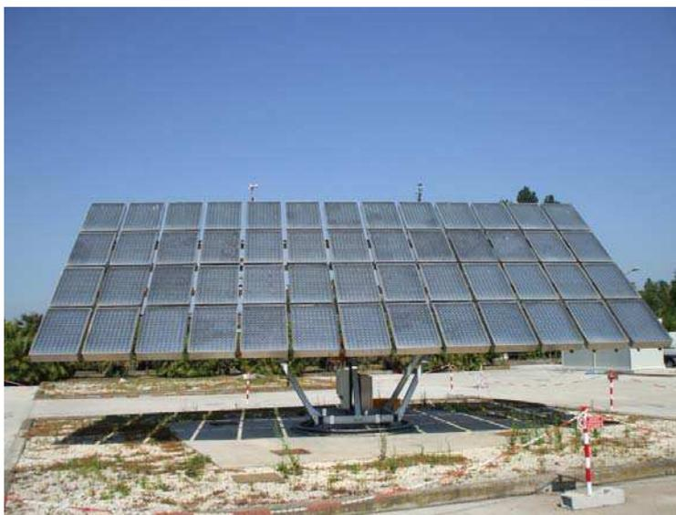
Fig. 14. CPV tracking system in Sun; installation of Rondine™ CPV modules on standard sun-tracker for flat plate modules in Sicily (South Italy). (Courtesy of CPower Srl – [www.cpower.it](http://www.cpower.it))
