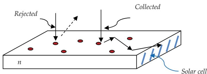
Fig. 7. Simplified drawn of a luminescent solar concentrator
