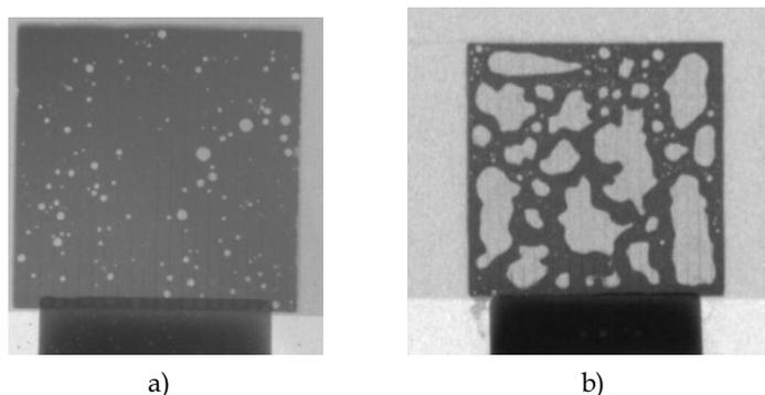
Fig. 13. X-ray image of soldered solar cells – a) acceptable soldering with <math><5\%</math> of voids area; b) unacceptable soldering, with high fraction of voids under the cell
