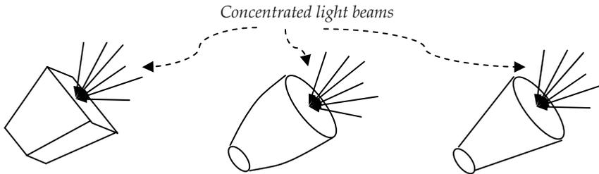
Fig. 5. Examples of geometries for simple secondary concentrators
