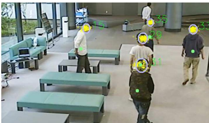
Fig. 4. Tracking results by the combination of multi-camera and LRF. The grey circles indicate head tracking result and the yellow dot clouds show hypotheses. The green dots on the bodies indicate base LRF tracking results.
