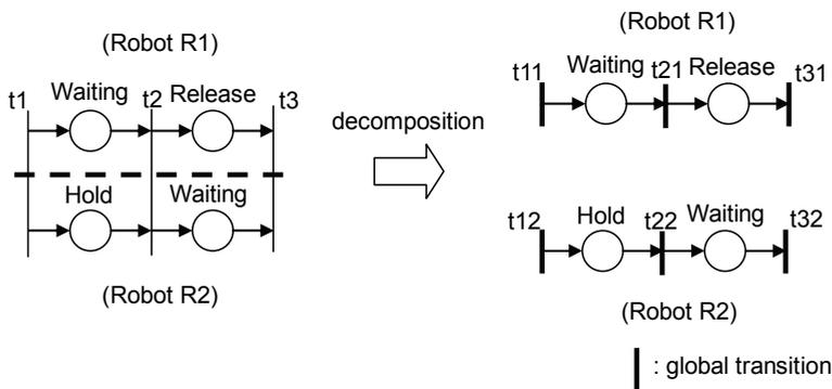
Fig. 13. Decomposition of transitions in "Hand over" operation
