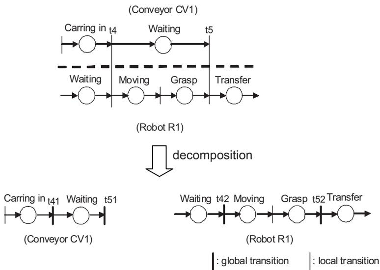
Fig. 14. Decomposition of transitions in the "Loading" operation
