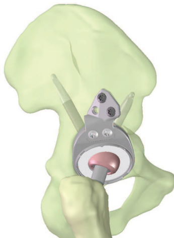
Fig. 7. CAD-prototype of the newly developed acetabular cup revision system with modular adaptable lateral flap and fixation pegs
