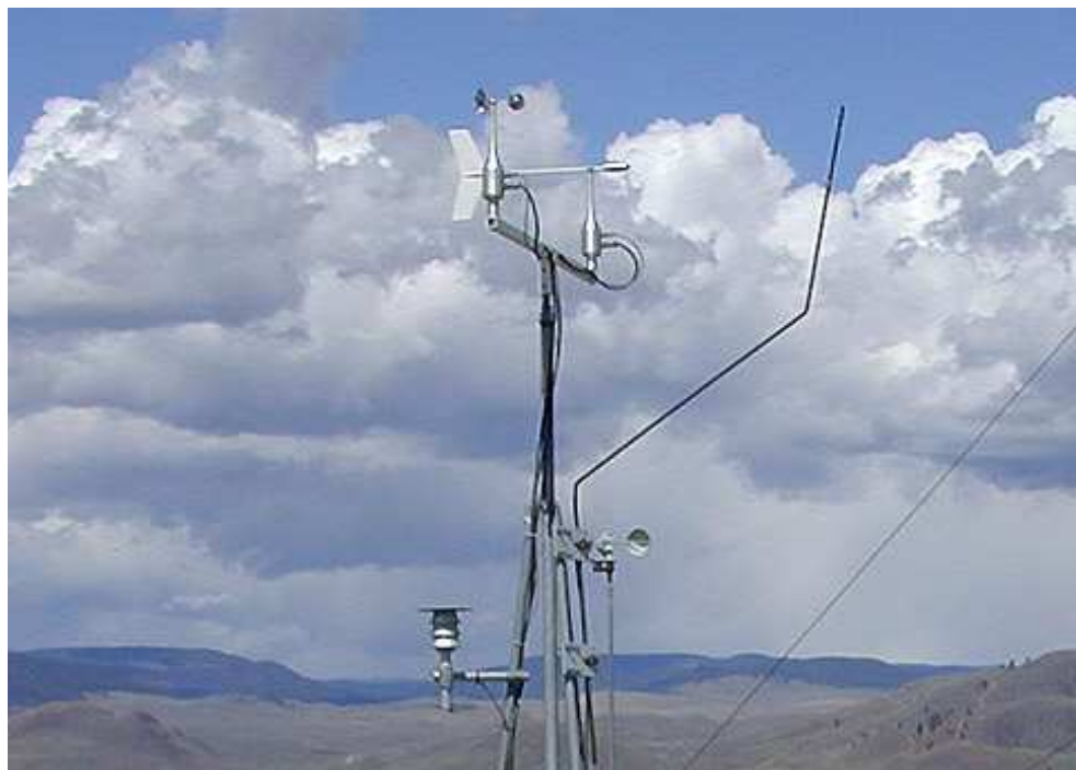
Fig. 2. Anemometer used to measure wind speed and direction (Pidwirny, 2006)
