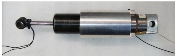
Fig. 3. Photograph of self-sensing MR damper prototype
