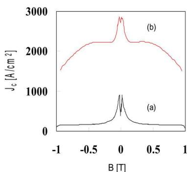
Fig. 10. The dependence of current density on magnetic flux density. Sample (a) was prepared with  $\text{YBa}_2\text{Cu}_3\text{O}_{7-x}$  powder made by conventional sintering method. Sample (b) was prepared with  $\text{YBa}_2\text{Cu}_3\text{O}_{7-x}$  powder made by MPMQ method.
