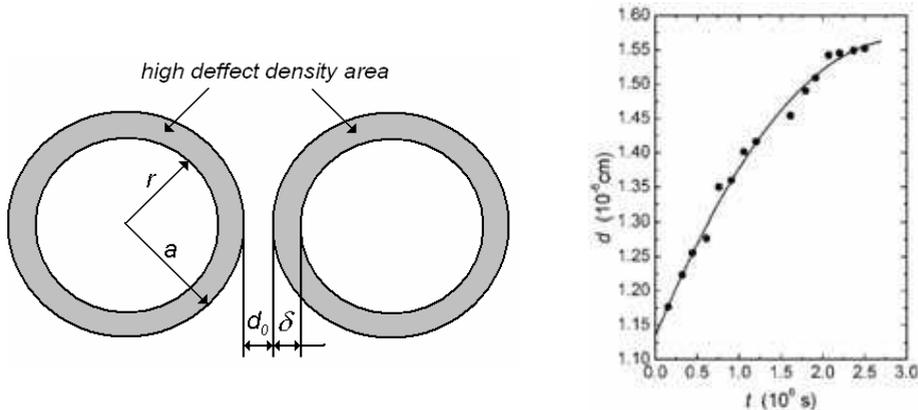
Fig. 18. Schematic representation of the YBCO superconducting weak intergrain linking: intragrain defect distribution and the intergrain junction thickness  $d$  (left). Evolution of the superconductive junction thickness  $d$  with the  $^{57}\text{Co}$  irradiation time (right).
