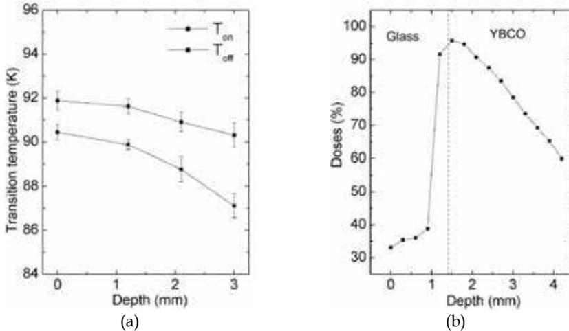
Fig. 13. (a) In-depth  $T_c$  profile in a  $^{137}\text{Cs}$  gamma irradiated YBCO sample,  $T_c$  measurements were performed through step by step sample polishing. (b) Energy deposition distribution calculated for a model irradiation experiment by means of the EGS-4 code (Leyva et al., 2002a).
