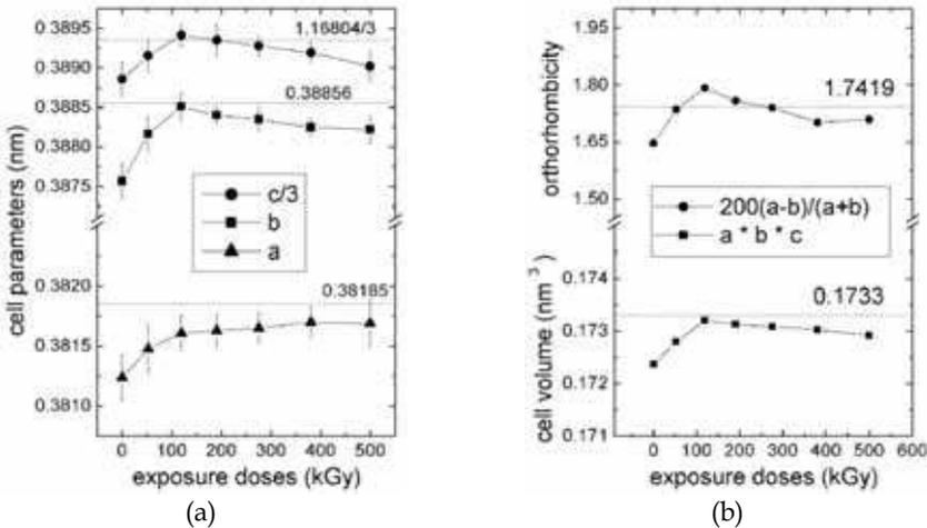
Fig. 10. <sup>60</sup>Co -  $\gamma$  dose exposition dependence of the YBCO elementary cell parameters, volume and orthorhombicity behaviors measured by X-Ray Diffraction. (a) Orthorhombic cell lengths a, b and c. (b) Elementary volume and orthorhombicity. Dashed lines represent the presupposed optimum values of YBCO cell parameters, volume and orthorhombicity.
