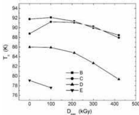
Fig. 14. YBCO superconducting transition temperature  $T_c$  dependence on  $^{60}\text{Co}$  induced gamma ray exposition doses at different initial non-stoichiometric parameter  $\delta$  values, 0.05, 0.09, 0.18 and 0.23 for A, B, C and D curves respectively.
