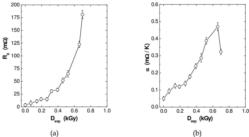
Fig. 17. Exposition dose dependence of (a) residual resistivity  $R_0$  in ( $\text{m}\Omega$ ) and (b) thermal electrical resistivity coefficient  $\alpha$  ( $\text{m}\Omega\text{K}^{-1}$ ) of  $^{57}\text{Co}$  irradiated YBCO ceramic samples at room temperature.
