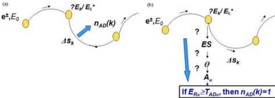
Fig. 3. (a) Fukuya’s treatment of atom displacements processes (Fukuya & Kimura, 2003). (b) New MCSAD approach (Cruz et al., 2008).  $E_k$  denotes the electron kinetic energy;  $n_{dpa}$  is the number of atom displacements events. Solid bold balls represent the occurrence of single scattering events (Elastic Scattering, Moeller or Bremsstrahlung).
