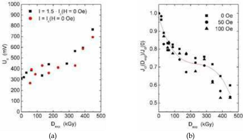
Fig. 15. Transport properties in a YBCO thick film exposed to  $^{60}\text{Co}$  gamma radiation. Vortex pinning energies (a) and superconducting electrical critical current (b) vs. exposition doses; the continuous curve is a visual guide. (Leyva et al, 1995)
