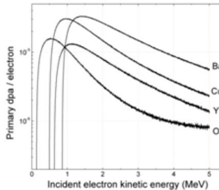
Fig. 4. Monte Carlo simulation of ES processes inducing Primary Knock-On Atomic Displacements in  $\text{YBa}_2\text{Cu}_3\text{O}_{7.5}$  depending on electron initial energy at a given discrete event.
