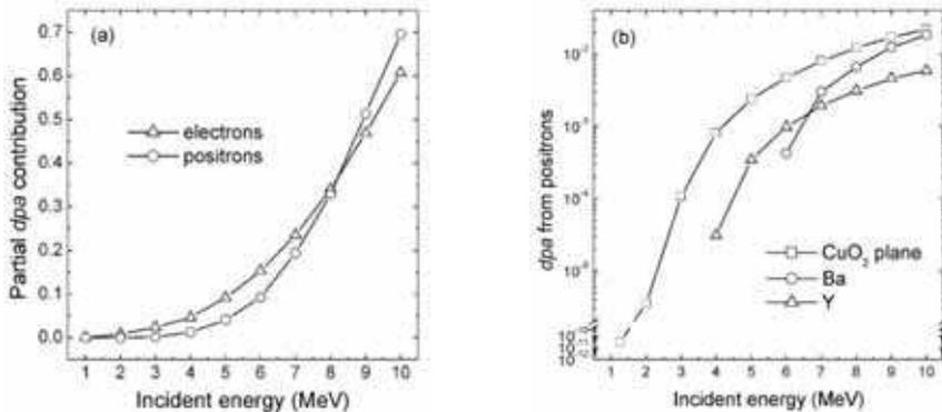
Fig. 6. (a) Number of *dpa* induced by electrons and positrons at different incident gamma energies. (b) Number of positrons *dpa* corresponding to each atom site at different incident gamma energies. All continuous lines are only visual guides.
