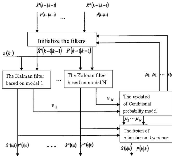
Fig. 3.3 Algorithm Flow of the Interacting Multiple Model
