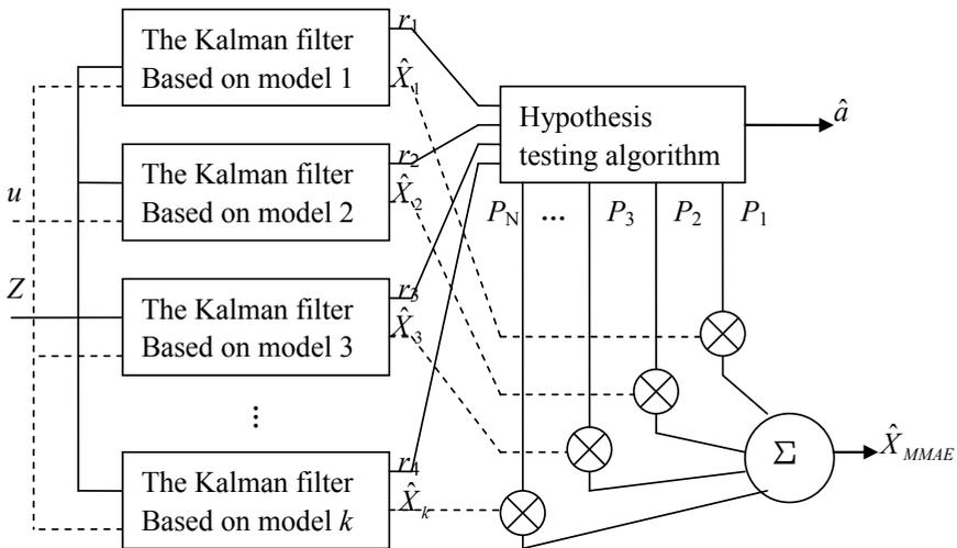
Fig. 3.2 Structure Diagram of Multiple-Model Adaptive Estimators
