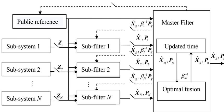
Fig. 4.1 Structure Indication of the Combined Filter
