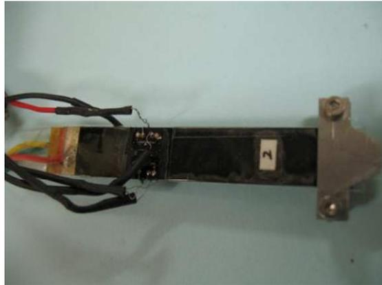
Fig. 9. Macle piezoelectric ceramics affixed with strain gages
