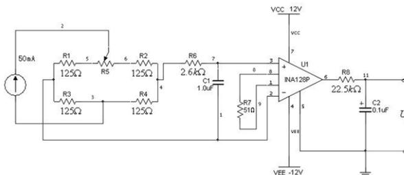
Fig. 7. (b) Amplification and filtering circuit diagram
