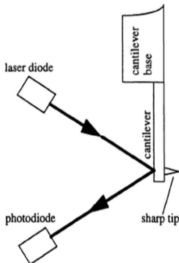
Fig. 3. Basic structure of optical force sensing system
