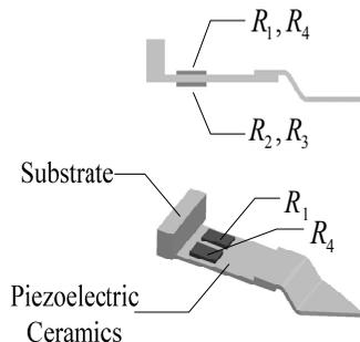
Fig. 2. Affixed position of semiconductor strain gages
