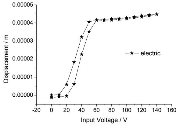
(c) Displacement obtained from amplification filtering circuit
