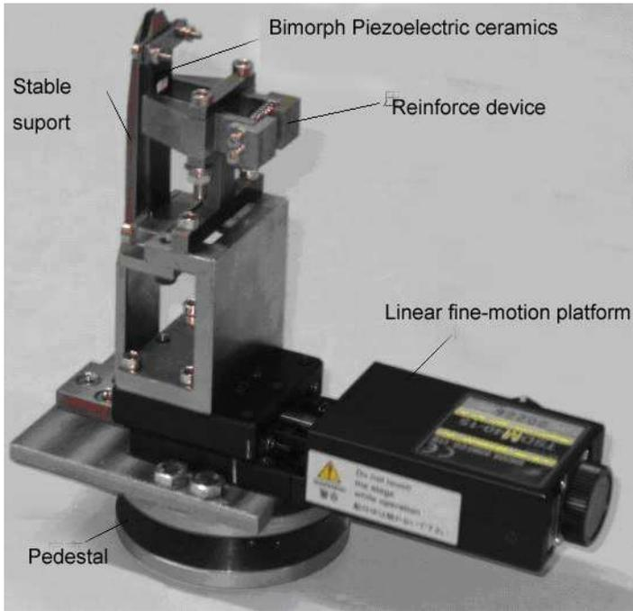
Fig. 5. Microgripper based on made piezoelectric ceramics
