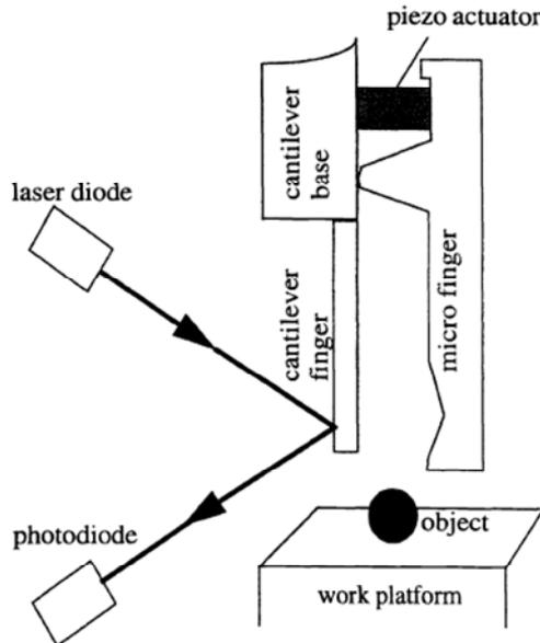
Fig. 4. Principle of microgripper with built-in optical force sensor
