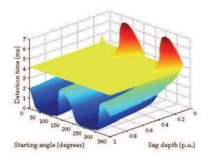
Fig. 16. Probability that sags and interruptions are detected in less than a quarter of cycle, with the KF-RMS algorithm.
