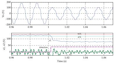
Fig. 7. Estimation of the rms value of a distorted supply voltage with the KF. The detection of a 0.4*p.u*. sag is also shown.
