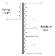
Fig. 4. Transformer with electronic tap changers.
