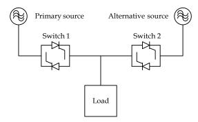
Fig. 2. Static transfer switch (STS).
