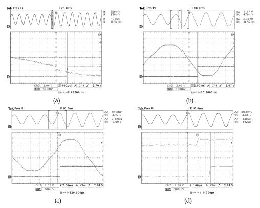
Fig. 21. Experimental detection times of the KF-RMS algorithm for swells. a) 0.4p.u. swell at 224°,  $t_d = 496\mu s$ . b) 0.4p.u. swell at 153°,  $t_d = 3.36ms$ . c) 0.4p.u. swell at 0°,  $t_d = 2.12ms$ . d) 0.4p.u. swell at 80°,  $t_d = 140\mu s$ .
