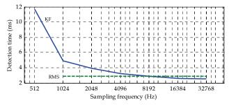
Fig. 18. Dependence of the detection time of KF and RMS methods on the variation of the sampling frequency, for a 0.4*p.u.* rectangular sag starting at electrical 0°.
