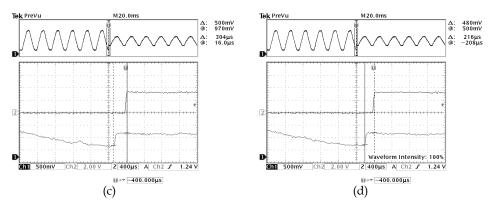
Fig. 20. Experimental detection times of the KF-RMS algorithm for sags. a) 0.4p.u. sag at 80°,  $t_d = 288 \mu s$ . b) 0.5p.u. sag at 170°,  $t_d = 3.12 m s$ . c) 0.5p.u. sag at 260°,  $t_d = 304 \mu s$ . d) 0.5p.u. sag at 270°,  $t_d = 216 \mu s$ .
