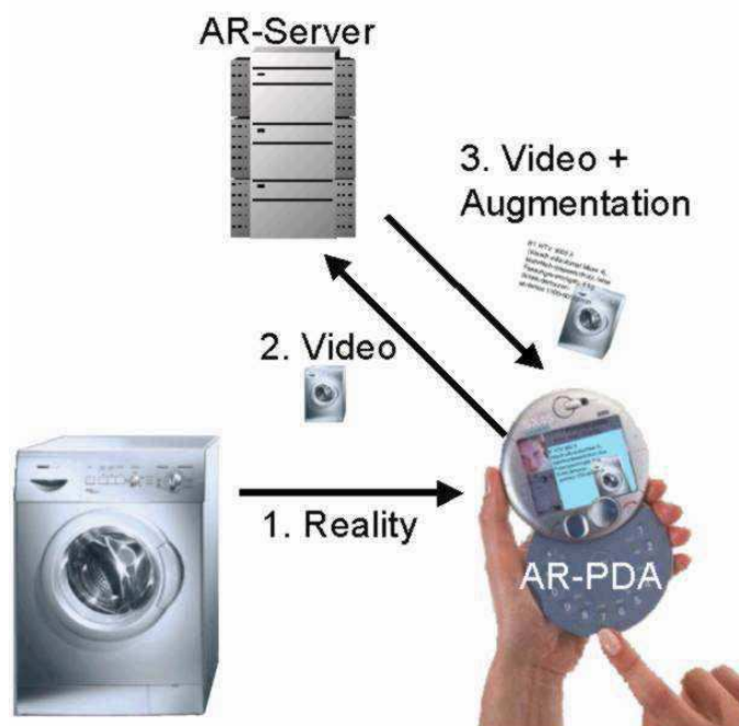
Fig. 3. Mobile mixed reality: Interaction of mobile device with backend AR server with wireless connectivity.
