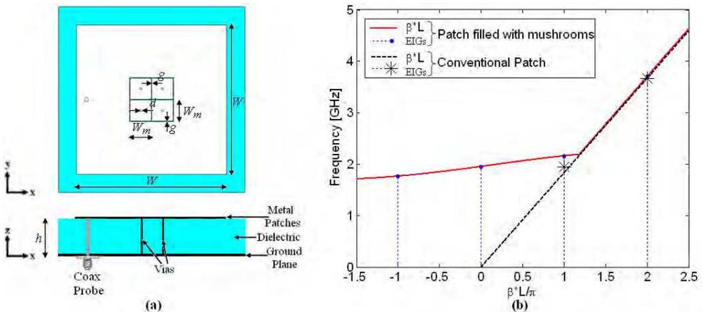
Fig. 19. Dual-frequency antenna based on a microstrip patch filled with LH cells. (a) Sketch of the antenna. (b) Electrical length ( $\beta L$ ) and eigenfrequencies (EIGs) of the resonant modes of the proposed antenna (solid red line). The same information for the conventional patch antenna is also plotted in the dashed line.
