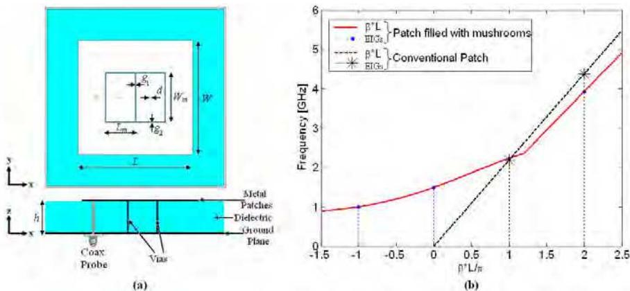
Fig. 15. Triple-frequency and dual-mode antenna based on a microstrip patch filled with LH cells. (a) Sketch of the antenna. (b) Electrical length ( $\beta L$ ) and eigenfrequencies (EIGs) of the resonant modes of the proposed antenna (solid red line). The same information for the conventional patch antenna is also plotted in the dashed line.
