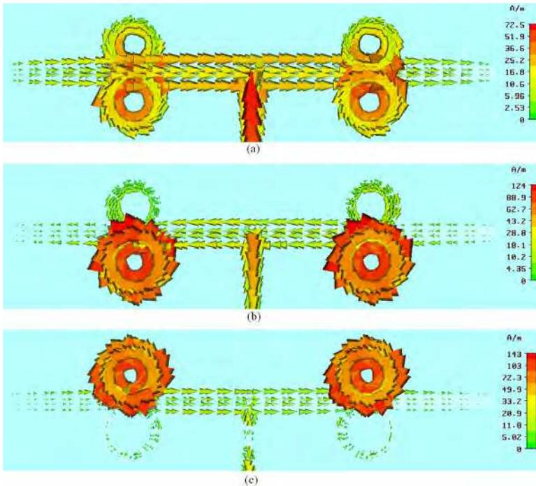
Fig. 13. Currents on the triple-frequency printed dipole loaded with SRRs. (a)  $f_1$  (fundamental frequency of the unloaded dipole). (b)  $f_2$  (resonant frequency of the SRRs with  $R_2$ ). (c)  $f_3$  (resonant frequency of the SRRs with  $R_1$ ).
