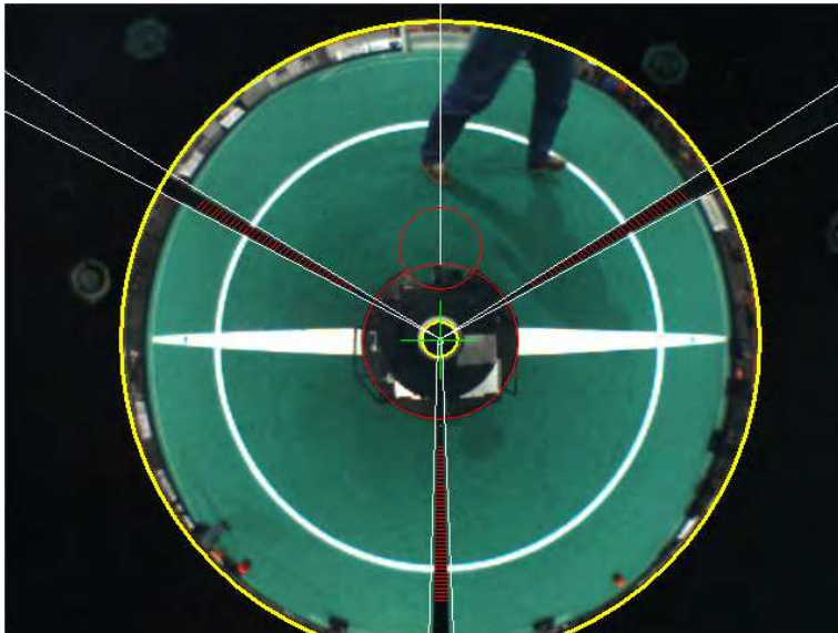
Fig. 10. Automatic extraction of main image features, while robot is standing at the center of a MSL middle field circle.
