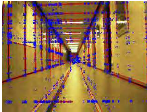
Fig. 7. The illustration of the vanishing point extraction. The extracted lines are shown in red, the vanishing point candidates are shown in blue and the green cross at the center is the detected vanishing point.
