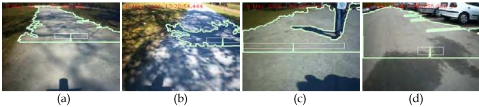
Fig. 14. Shadows and road markings at the limits of the vision sensor capabilities. Unfocused shadows like in (a) are handled reasonably well, but if the shadows are more focused as in (b) the result is of little or no use. Hard shadows as in (c) and road markings as the white markings in a parking lot in (d) are handled as obstacles.
