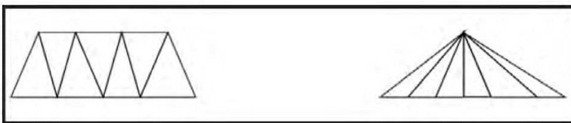
Fig. 3. Triangle strips and triangle fans can reduce the number of redundant points.
