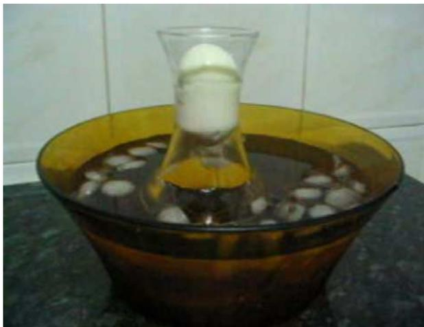
Fig. 2. Egg moving downwards by pressure difference
