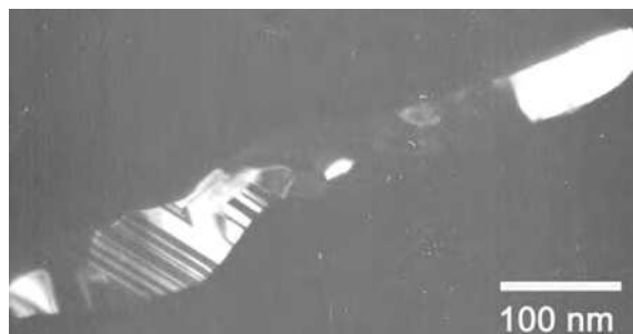
Fig. 5. TEM dark field image of a nanowire grown for approximately 1/3 of the time of the nanowires in Fig. 1(a). Twin defects can be observed. The 111 reflection was used to form the image. Taken from (Selvig et al. , 2006).
