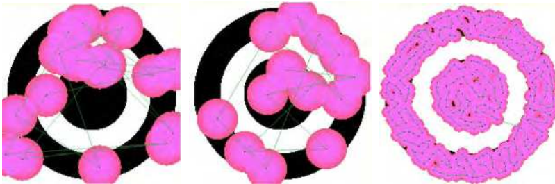
Fig. 10. ParaSOM in action: a) randomly initialized with a predetermined number of neurons; b) the network position at iteration 25; c) the network at iteration 500
