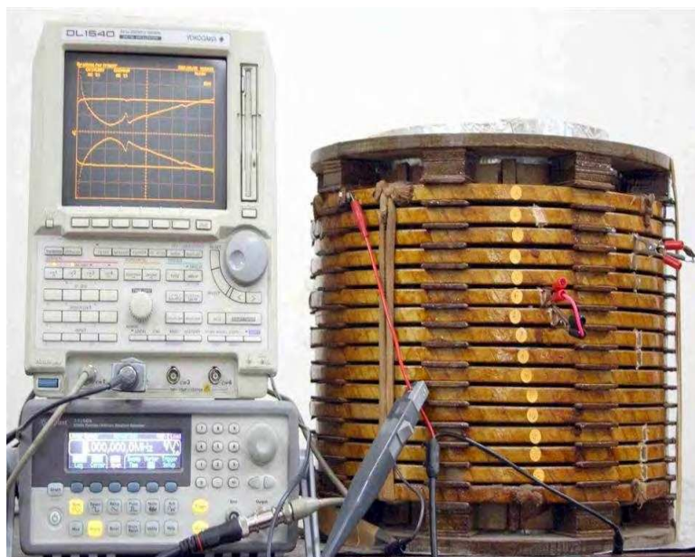
Fig. 2. Experimental arrangement for frequency response measurements on an interleaved winding
