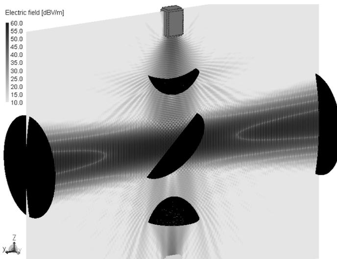
Fig. 8. The full model of Fabry-Perot resonator
