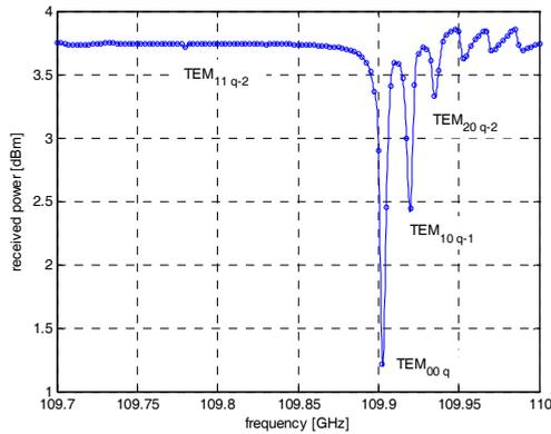
Fig. 6. Higher-order modes around frequency of 110 GHz
