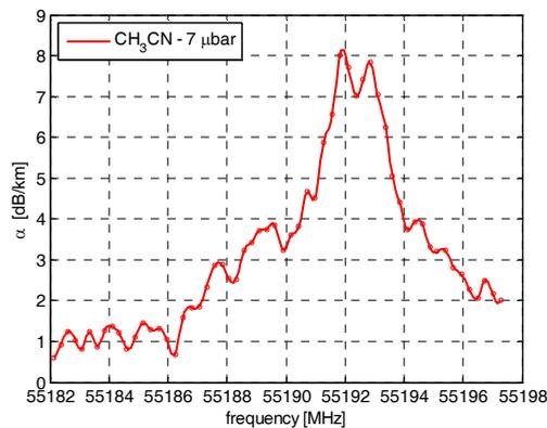
Fig. 14. Gas absorption loss of acetonitrile  $\text{CH}_3\text{CN}$  under pressure of 7  $\mu\text{bar}$
