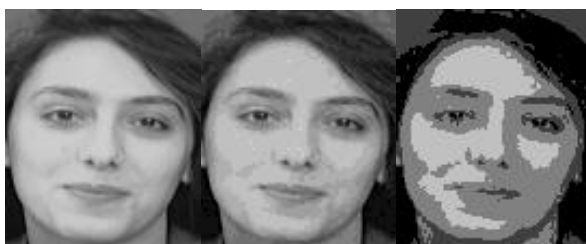
Fig. 8. Bit quantization: left most is the original 8 bit image (from ORL database), next two are 4 bit and 2 bit representations respectively [Mandal et al., 2007].
