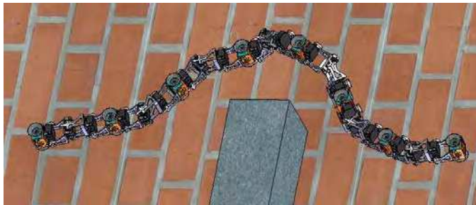
Fig. 3. 3D-animation of the planned robotic caterpillar
