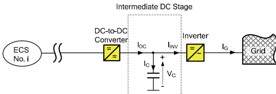
Fig. 15. System overview of the intermediate DC stage.
