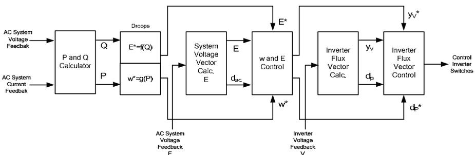
Fig. 8. Inverter control scheme (M. C. Chandorkar 1993).
