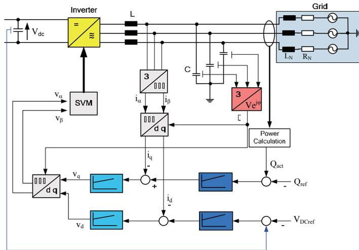
Fig. 24. Q-controlled inverter in grid parallel mode.
