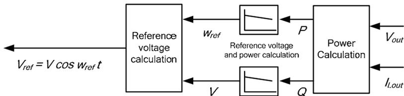
Fig. 7. Reference voltage and power calculation (C.-C. Hua).
