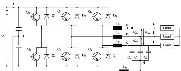
Fig. 20. Three-leg inverter with a neutral point.
