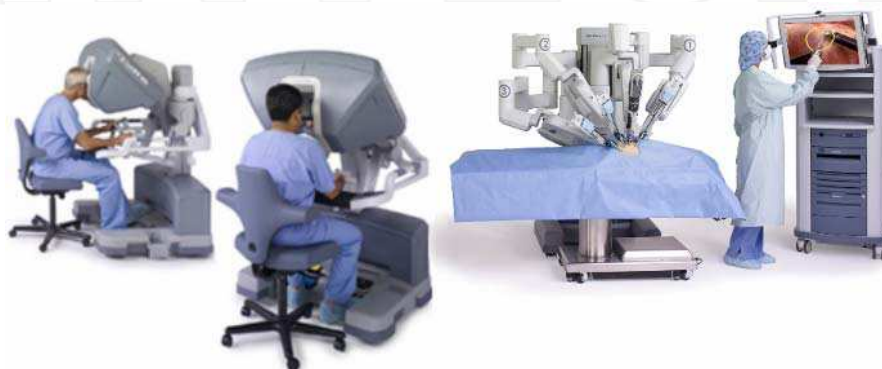
Fig. 2. Master controllers and the patient side manipulators of the new da Vinci Si surgical system. (Photo: Intuitive Surgical Inc.)
