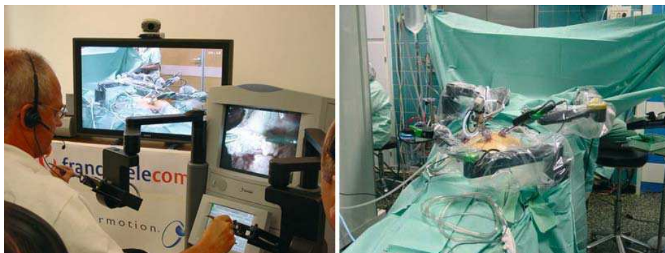
Fig. 4. The Zeus robot during the first intercontinental surgery, the colecystectomy was performed on the patient in Strasbourg from New York. (Photo: IRCAD)
