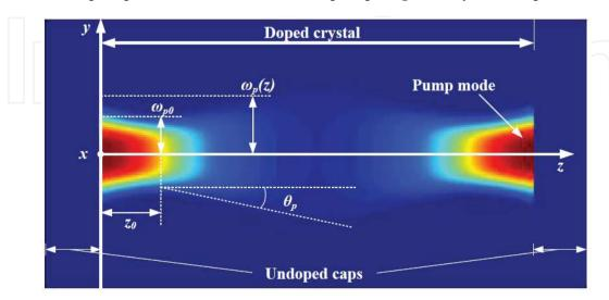
Figure 7. Pump modeling of the dual-end-pumped geometry [44].
