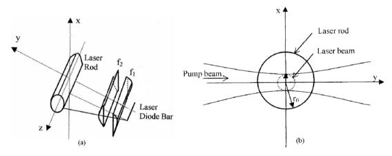
Figure 3. side pumping geometry; a) Pumping of a laser rod by one module, b) end view of side pumping geometry [27].
