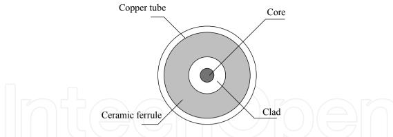
Figure 22. Geometry of modeled fiber laser
