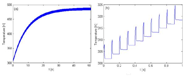
Figure 26. a) time evaluation of temperature at the end surface of fiber, b) enlarged drawings of the part of graph a which shows regular fluctuations in temperature profile [73].
