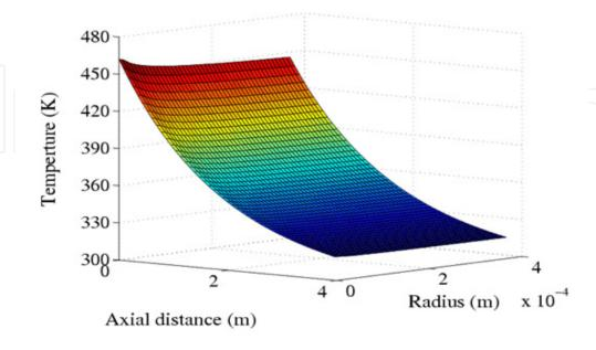
Figure 20. Temperature distribution in r-z plane for the double clad ZBLAN fiber laser [70].
