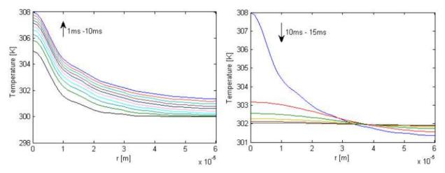
Figure 25. a) radial temperature distribution inside fiber laser at the pump facet during the first pulse pump time, b) reduction of temperature generated by the first pulse during 5ms [73].
