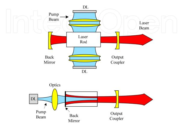
Figure 1. Simple drawing for two common pumping methods of solid state laser gain medium; a) side pumping b) end pumping. The blue color used for marking the pump light carrying energy from laser diode to the gain medium, and the red beam concerns to the laser resonator mode.
