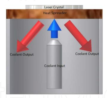
Figure 12. Schematic diagram of jet impingement cooling system for thin disk laser [54]
