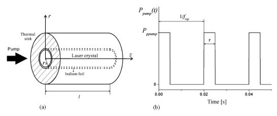
**Figure 8.** a) simple drawing of laser rod which is surrounded by a cylindrical heat sink, b) time variation of pump power [46]
