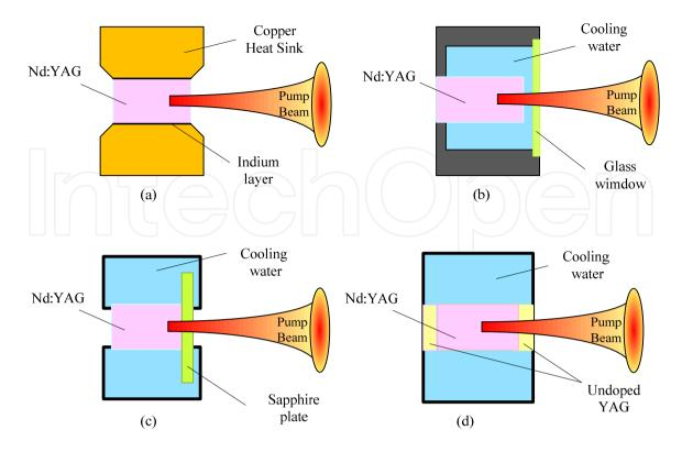
**Figure 6.** Different cooling configurations in end pumped systems. In these geometries the pumped surface (a) uncooled, (b) water cooled, (c) sapphire cold plate cooled, (d) undoped cap rod [33]. The figures are repainted in color version just for better realization.
