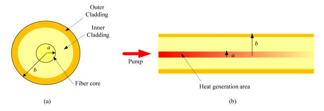
**Figure 19.** End (a) and side (b) view of circular fiber laser. Absorption of pump power inside the fiber core causes heat generation which reduces exponentially along the fiber axis [70].
