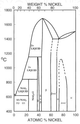
Figure 3. Phase diagram of Ni-Al alloy
