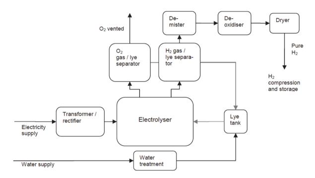
**Figure 1.** Schematic diagram of an alkaline electrolyzer [4]
