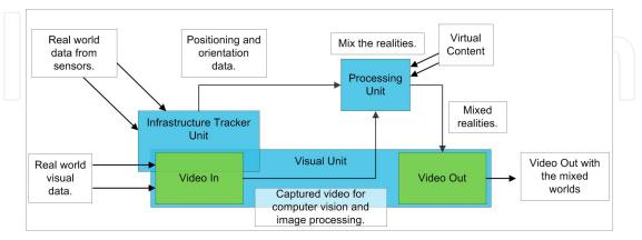
Figure 1. Augmented Reality Systems (ARS) standard design.
