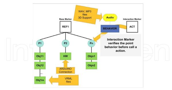
Figure 9. basAR Data Structure.
