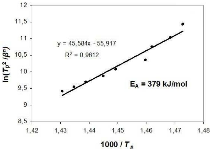
Fig. 24. The Kissinger plots for determining  $E_A$  associated with the first exotherm of the pre-nucleated 0.90TeO<sub>2</sub>-0.10WO<sub>3</sub> sample (Çelikbilek et al., 2011)
