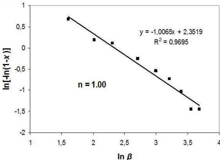
Fig. 25. The Ozawa plot for determining  $n$  associated with the first exotherm of the 0.90TeO<sub>2</sub>-0.10WO<sub>3</sub> sample pre-nucleated at 350 °C for 2 hours (Çelikbilek et al., 2011)
