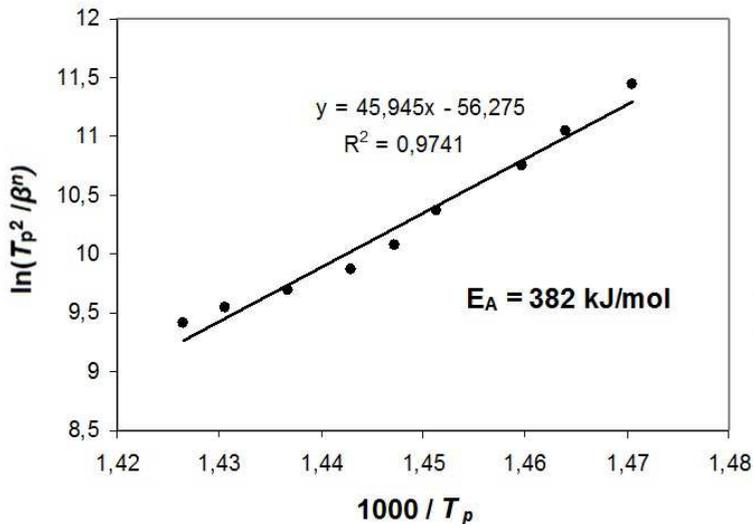
Fig. 26. The Kissinger plot for determining  $E_A$  associated with the first exotherm of the 0.90TeO<sub>2</sub>-0.10WO<sub>3</sub> sample pre-nucleated at 350 °C for 2 hours (Çelikbilek et al., 2011)
