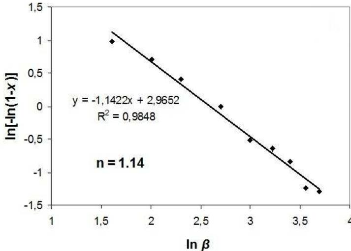
Fig. 23. The Ozawa plot for determining  $n$  associated with the first exotherm of the 0.90TeO<sub>2</sub>-0.10WO<sub>3</sub> sample (Çelikbilek et al., 2011)
