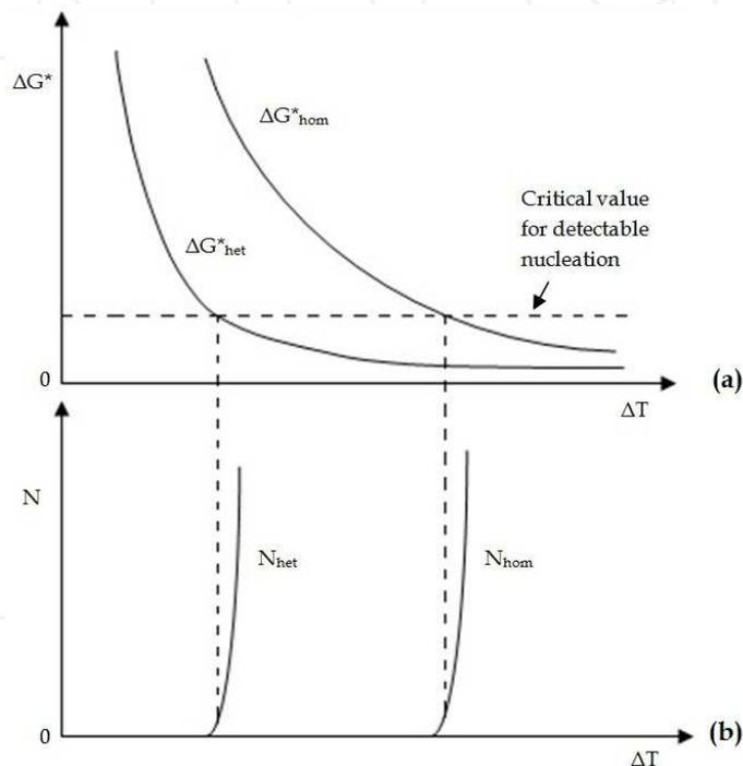
Fig. 7. (a) Variation of  $\Delta G^*$  with undercooling ( $\Delta T$ ) for homogeneous and heterogeneous nucleation, (b) The corresponding nucleation rates assuming the same critical value of  $\Delta G^*$  (Porter & Easterling, 1992)
