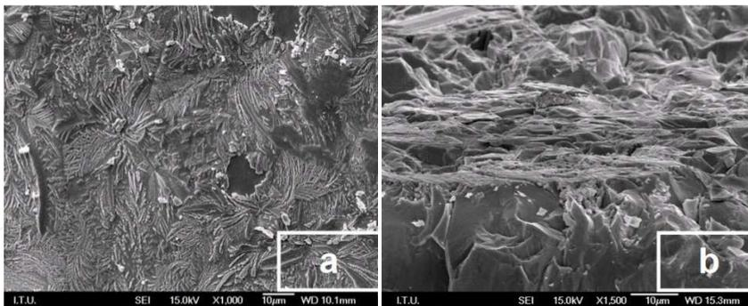
Fig. 27. SEM micrographs of the 0.90TeO<sub>2</sub>-0.10WO<sub>3</sub> sample heat-treated at 410 °C (a) surface, (b) cross-section (Çelikbilek et al., 2011)
