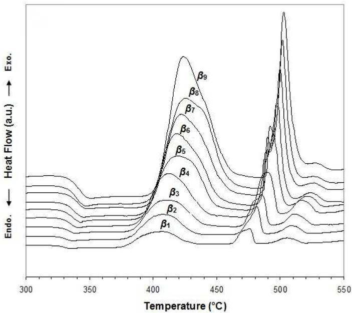
Fig. 22. DSC curves with heating rate  $\beta$  (5, 7.5, 10, 15, 20, 25, 30, 35 and 40 °C/min) for 0.90TeO<sub>2</sub>-0.10WO<sub>3</sub> sample (Çelikkbilek et al., 2011)
