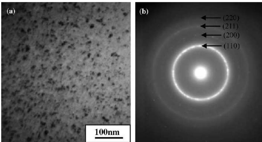
Fig. 31. Bright-field TEM image (a) and selected-area electron diffraction pattern, (b) of the  $\text{Ni}_{45}\text{Ti}_{23}\text{Zr}_{15}\text{Si}_5\text{Pd}_{12}$  bulk amorphous alloy annealed for 900 seconds at 840K (Qin, 2004)
